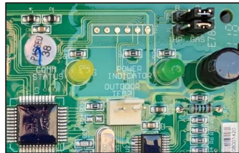
Figure 1 Survey Control LEDs
